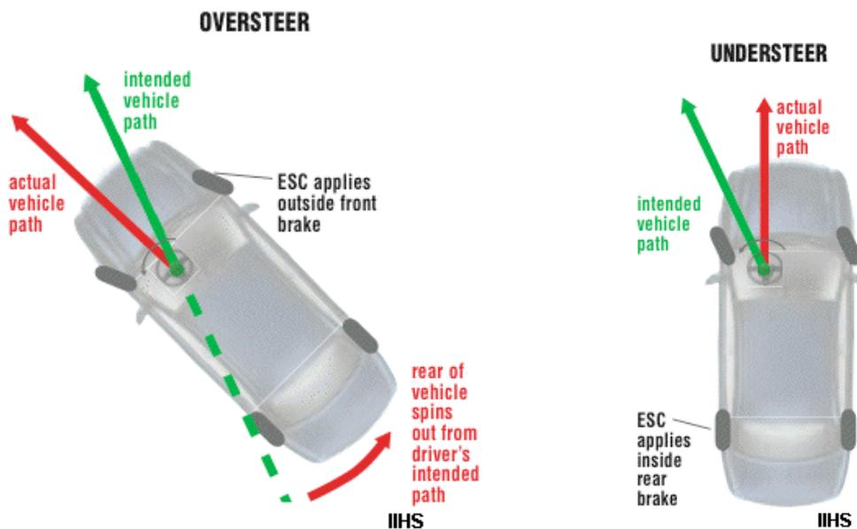
Figure 2. Methods of controlling oversteer and understeer
