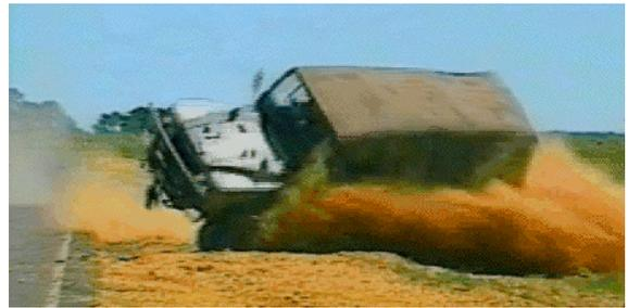
Figure 10. Example of off-road tripped rollover (credit: DV Experts)
