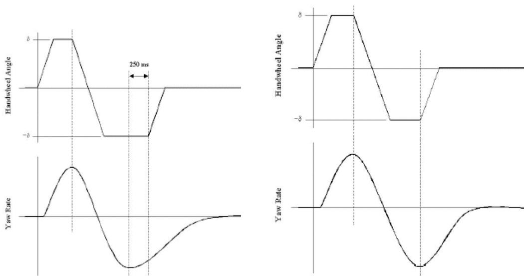
Figure 9. Steering Wheel Motion (Yaw Acceleration Tests)
