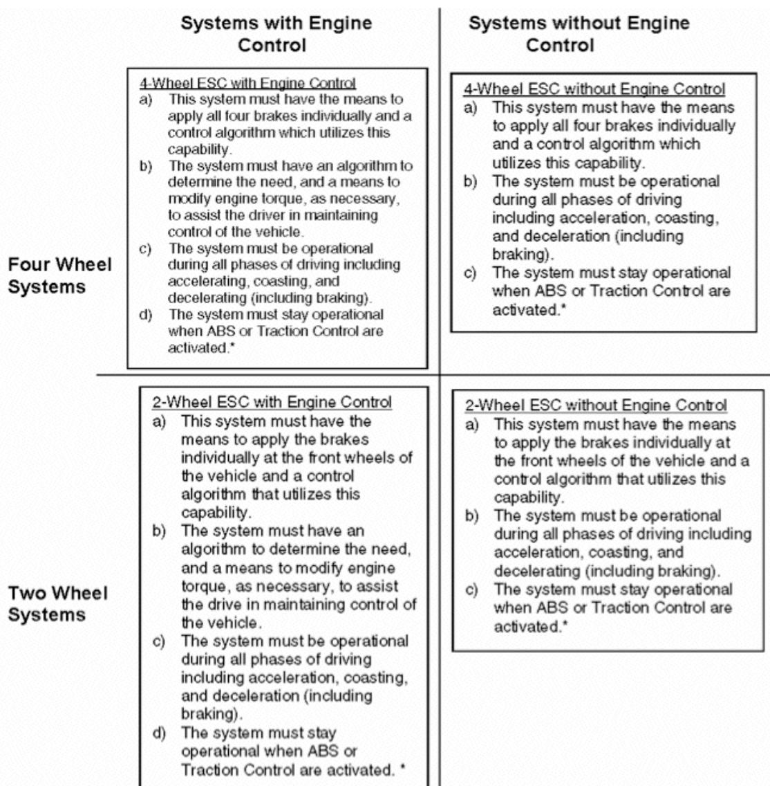
\*Some systems may have limited yaw control capability during ABS or Traction Control activation.
