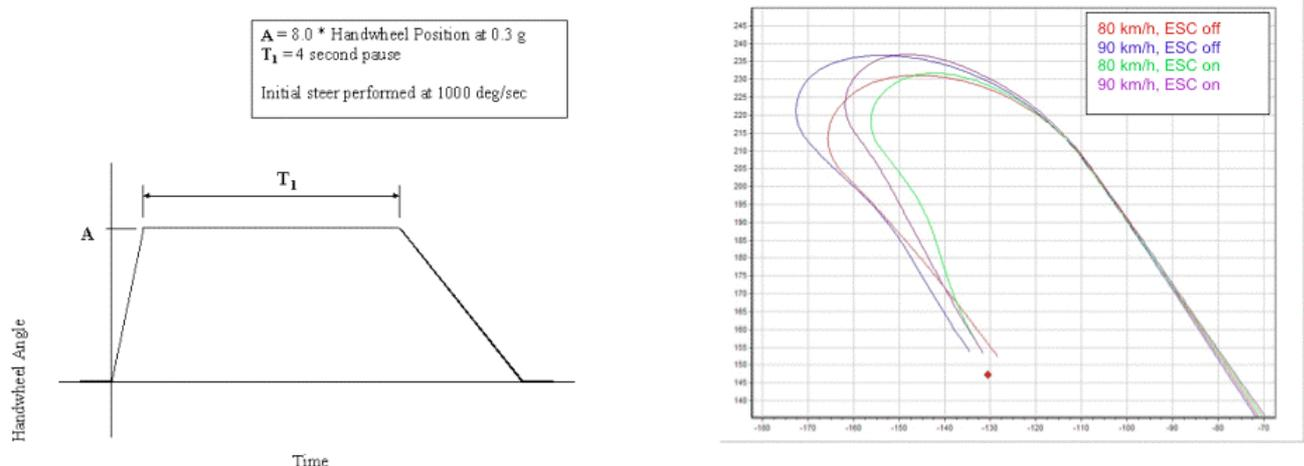
Figure 6. Steering input for J-turn test (ISO 7401) and typical vehicle path (Transport Canada)
